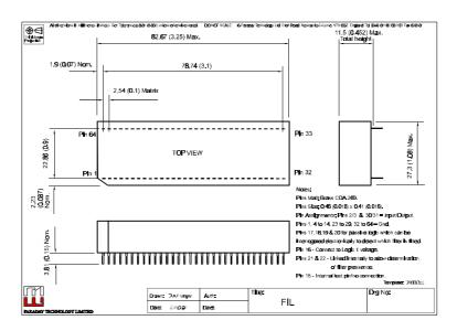
Note: For correct operation all the ground pins should be taken to a good earth plane.
