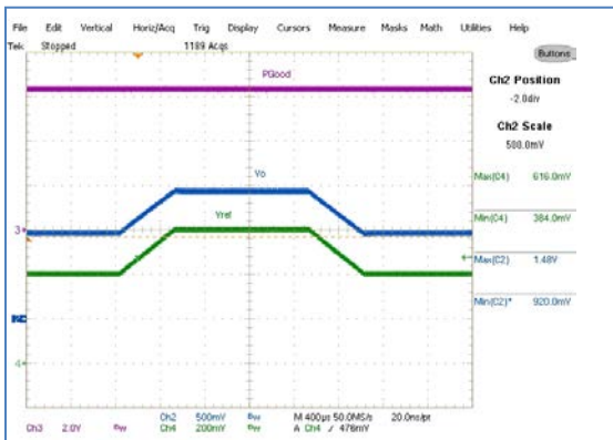
Figure 45: External frequency synchronization to 800KHz from free running 600KHz, Ch2- V_o , Ch3- LX , Ch4- Rt/Sync Voltage
