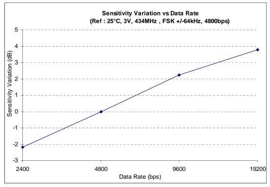
Figure 39. FSK Sensitivity Variation Versus Data Rate
