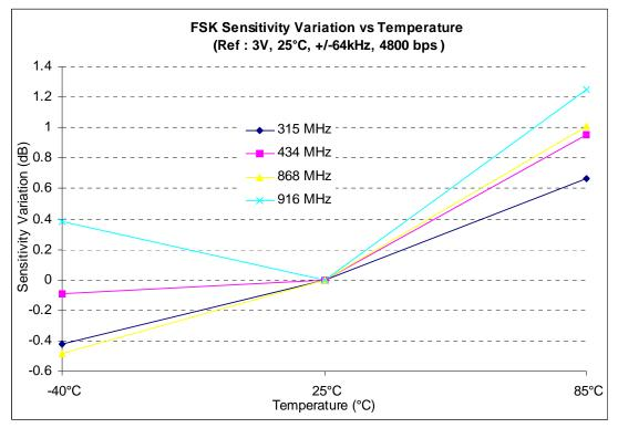
Figure 36. FSK Sensitivity Variation Versus Temperature
