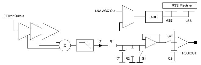
Figure 15. RSSI Simplified Block Diagram
