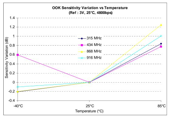
Figure 34. OOK Sensitivity Variation Versus Temperature
