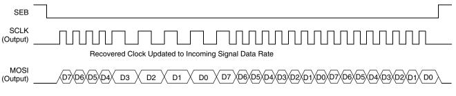
Figure 14. Typical Transfer in Receive Mode with Data Manager
