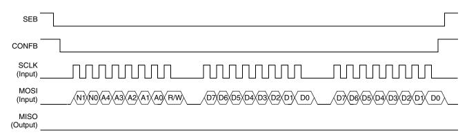
Figure 4. Write Operation in Configuration Mode (N[1:0] = 01)
