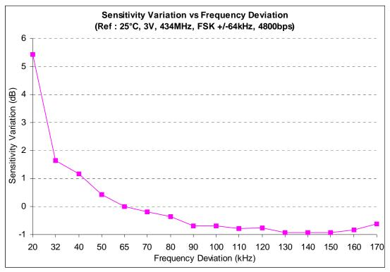
Figure 40. FSK Sensitivity Variation Versus Frequency Deviation
