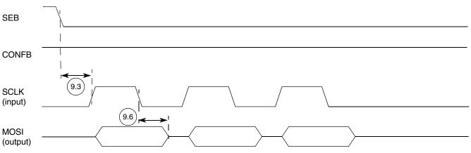
Figure 42. Digital Interface Timing Diagram in Receive Mode (DME = 1)
