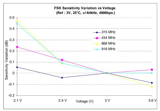
Figure 37. FSK Sensitivity Variation Versus Voltage
