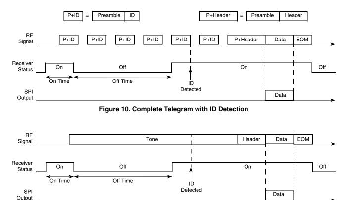
Figure 11. Complete Telegram with Tone Detection
