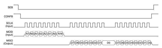
Figure 5. Read Operation in Configuration Mode (N[1:0] = 01)
