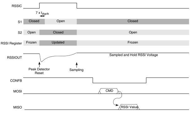
Figure 16. RSSI Operation in Sample Mode
