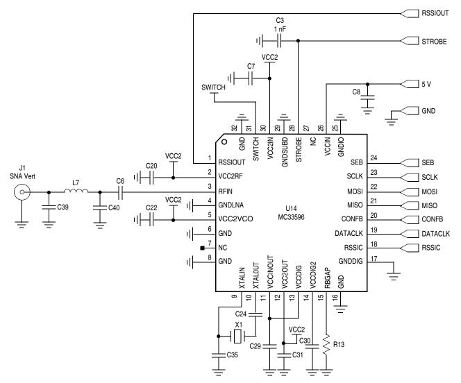
Figure 43. MC33596 Application Schematic (5 V)
