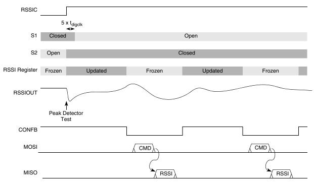
Figure 17. RSSI Operation in Continuous Mode
