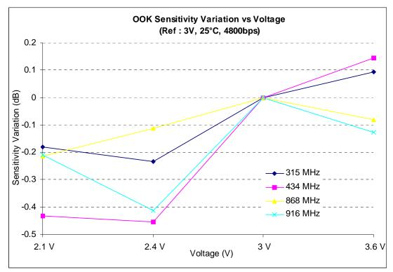
Figure 35. OOK Sensitivity Variation Versus Voltage
