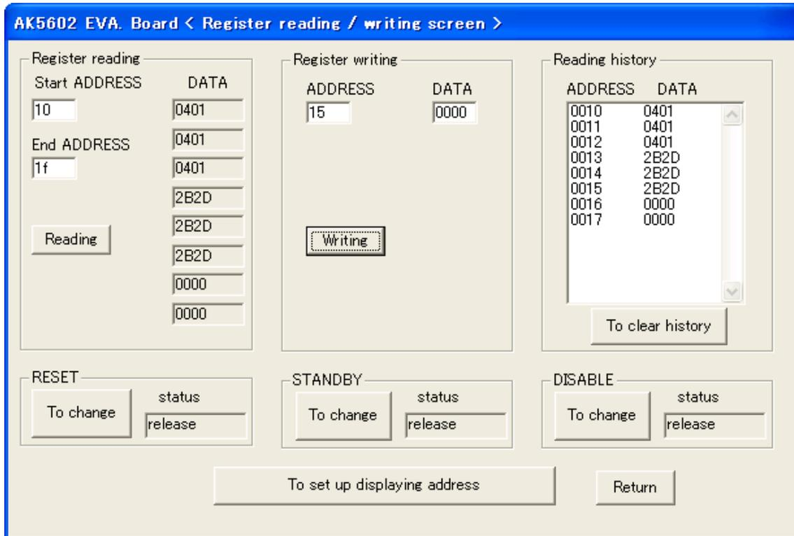
Before reading and writing AK5602A's registers properly, it is requested to change the state of RESET, STANDBY and DISABLE into "release" mode.
