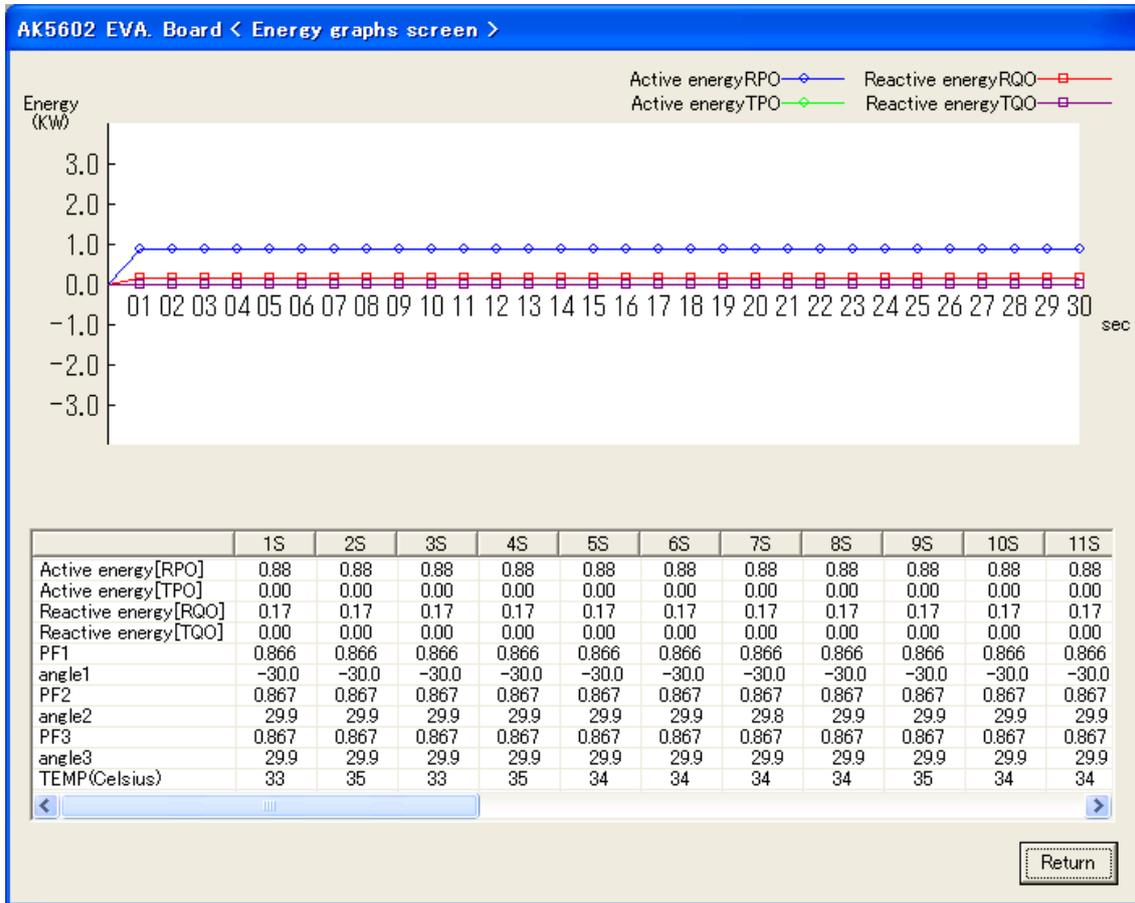
Based on the acquired data by the measurement, the numerical value and the graph of active energy and reactive energy are plotted. Furthermore, the numerical value of power factor, the phase angle between each current input and voltage input and the temperature of the LSI are also displayed.
