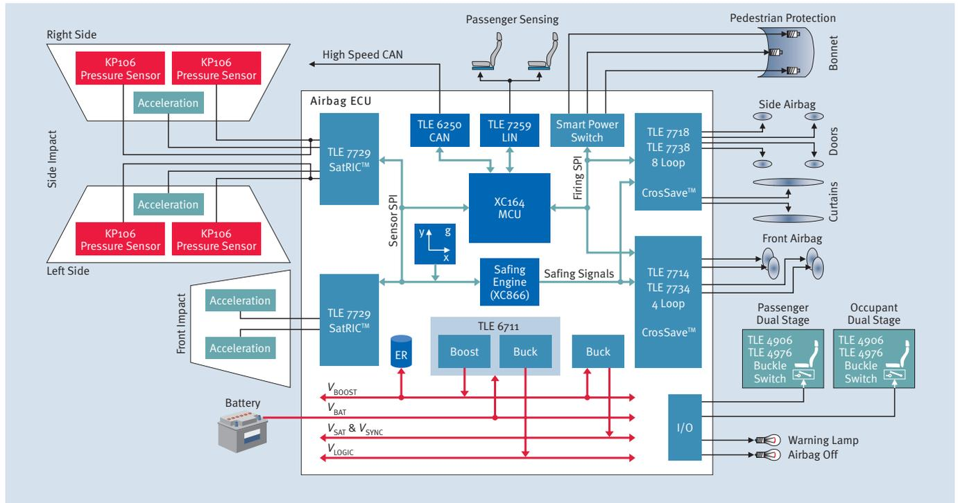
INFINEON TECHNOLOGIES offers an extensive product portfolio for occupant safety systems from micromachined sensors to smart power ICs and microcontrollers. The KP106 as an integrated pressure sensor systems for side crash detection, is a benchmark in terms of reliability and integration level.
