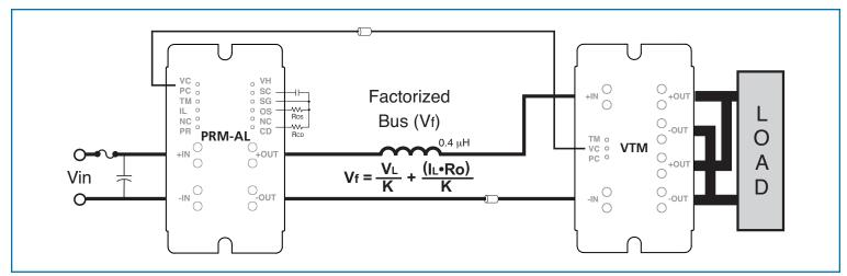
Figure 16 — Adaptive Loop compensation with soft start using the SC port.
