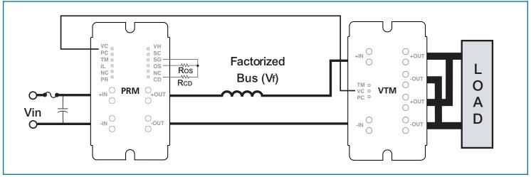
*Figure 15*— With Adaptive Loop control, the output of the VTM is regulated over the load current range with only a single interconnect between the PRM and VTM and without the need for isolation in the feedback path.
