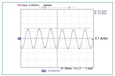
Figure 3 — Input reflected ripple current
