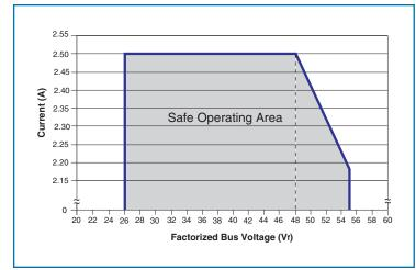
Figure 17 — PR024A480T012FP rating based on Factorized Bus voltage
