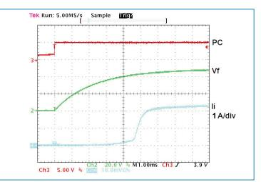
Figure 2 — Vf turn-on waveform with inrush current – PC enabled
