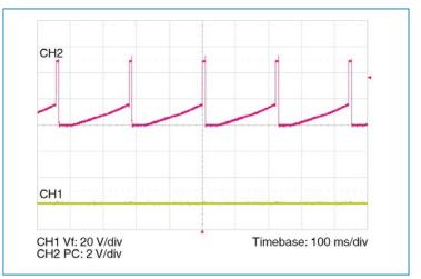
Figure 11 — PC during fault – frequency will vary as a function of line voltage
