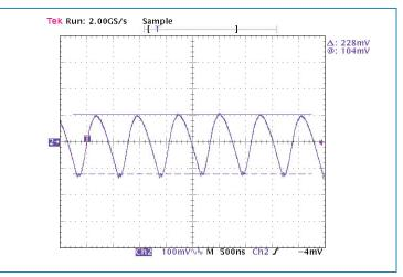
Figure 13 — Output ripple full load 10  $\mu$ F bypass capacitance
