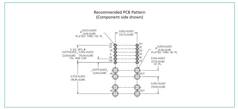
Figure 20 — PCB mounting specifications
