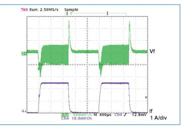
Figure 9 — Transient response; PRM alone 18 Vin, 0-2.5-0 A no load capacitance, local loop
