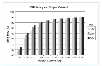
Figure 6 — Efficiency vs. output current at 36 Vf
