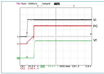
Figure 1 — Vf and PC response from power up
