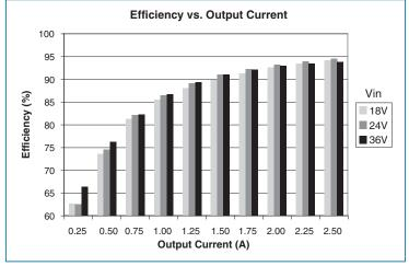
Figure 7 — Efficiency vs. output current at 26 Vf
