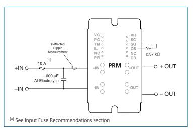
Figure 4 — Input filter capacitor recommendation
