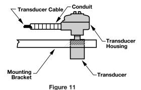
5. Tighten the conduit to the threads on the top of the transducer. Refer to Figure 9.
