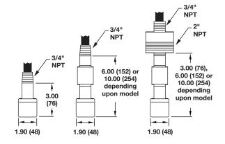
Figure 32 %" and 2" NPT Transducer without Housing
