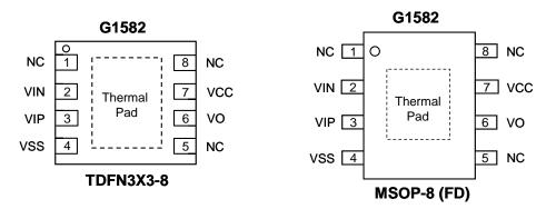
Note: Recommend connecting the Thermal Pad to the Pin#4 VSS for excellent power dissipation.
