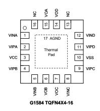
Note: Recommend connecting the Thermal Pad to the Pin#10 VSS for excellent power dissipation.
