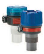
Echotel® Model 355 is a two-wire, loop-powered, non-contact ultrasonic transmitter that performs liquid level, volume, and open channel flow measurement. A powerful 60 kHz ultrasonic transducer and advanced digital signal processing is featured to reliably measure out to a 20 foot (6 meter) maximum range.
