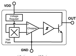
$\begin{array}{lll} \mbox{A Package} & \mbox{AT Package} \\ \mbox{Pin 1} - \mbox{V}_{\mbox{DD}} & \mbox{Pin 1} - \mbox{V}_{\mbox{DD}} \\ \mbox{Pin 2} - \mbox{GND} & \mbox{Pin 2} - \mbox{OUT} \\ \mbox{Pin 3} - \mbox{OUT} & \mbox{Pin 3} - \mbox{GND} \\ \end{array}$
