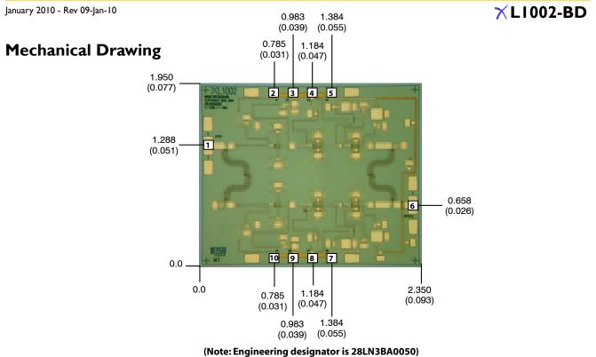
Units: millimeters (inches) Bond pad dimensions are shown to center of bond pad. Thickness: 0.115 + -0.010 (0.0045 + -0.0004), Backside is ground, Bond Pad/Backside Metallization: Gold All DC Bond Pads are  $0.100 \times 0.100 (0.004 \times 0.004)$ . All RF Bond Pads are  $0.100 \times 0.200 (0.004 \times 0.008)$  Bond pad centers are approximately 0.109 (0.004) from the edge of the chip. Dicing tolerance: +/-0.005 (+/-0.0002). Approximate weight: 2.838 mg.
