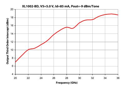
**Note** [1] **Measurements** – On-Wafer data has been taken using bias conditions as shown. Measurements are referenced 150 um in from RF In/Out pad edge. For optimum performance Mimix T-pad transition is recommended. For additional information see the Mimix "T-Pad Transition" application note.
