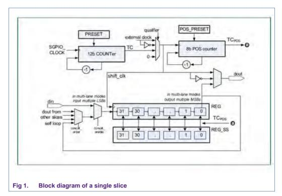
The slice's shift clock can be sourced from the SGPIO peripheral clock (SGPIO\_CLOCK). Please refer to Fig 2 below to understand SGPIO\_CLOCK's base clock, and section 5.1 for more SGPIO\_CLOCK setup.
