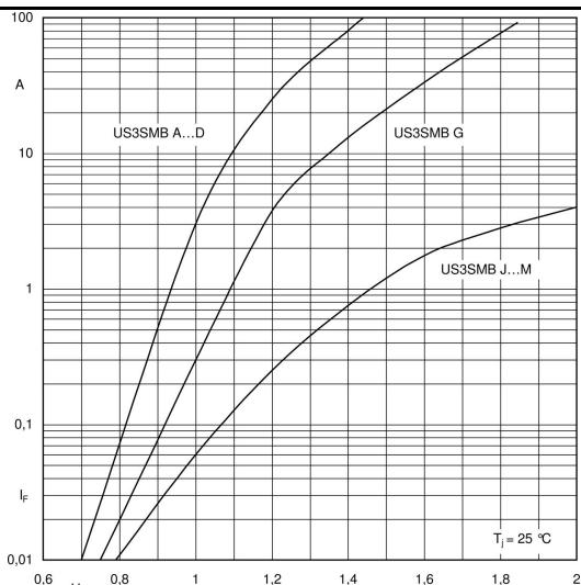
Fig. 1 Forward characteristics (typical values)
