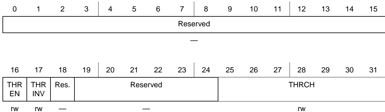
Figure 5-15. Threshold Control Register (TRCx, x = [0..3])
