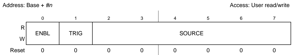
Figure 17-2. Channel Configuration Registers (CHCONFIG#n)
