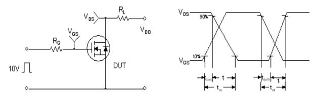
**Unclamped Inductive Switching Test Circuit & Waveforms**
