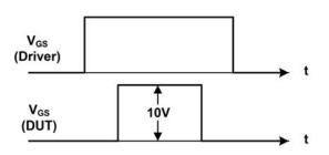
$$Qsync = \frac{1}{R_G} \cdot \int V_{R_G}(t) dt$$
