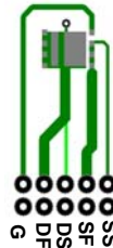
d. 120\text{ }^\circ\text{C/W} when mounted on a minimum pad of 2 oz copper
