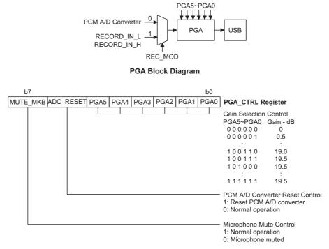
Programmable Gain Amplifier Control Register – PGA\_CTRL
