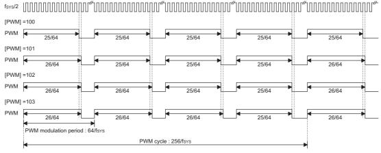
(6+2) PWM Mode Output Waveform
