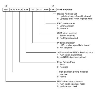
Serial Interface Setup Register – SIES
