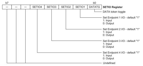
USB Endpoint Setup IN/OUT Pipe Register - SETIO
