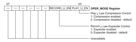
**Operation Mode Control Register – OPER\_MODE**
