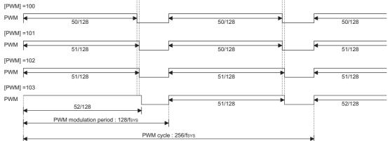
(7+1) PWM Mode Output Waveform
