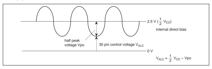
When ALC operation voltage is -5 dBV (at  $V_{CC} = 5$  V)
