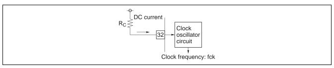
Note: The delay time (Td) for echo is determined by the clock frequency (fck).
