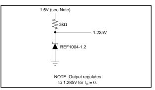
FIGURE 3. 1.2V Reference from 1.5V Battery.
