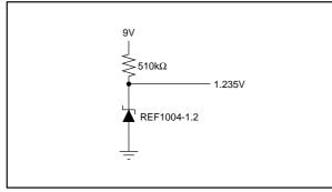
FIGURE2. Micropower Reference from 9V Battery.
