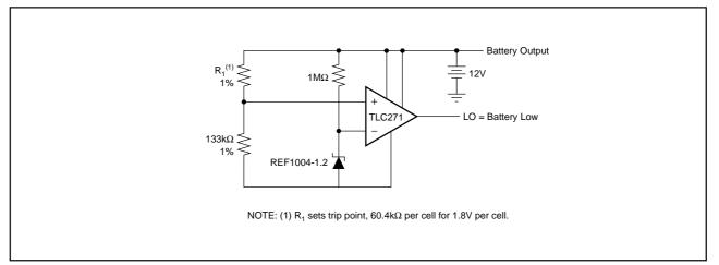
FIGURE 5. Lead-Acid Low-Battery-Voltage Detector.
