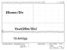
Fig.47 Output ripple 4 (VCC=12V, Io=170mA)
