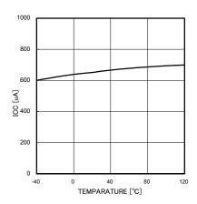
Fig.19. Circuit current temperature property
