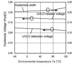
Fig.9. UVLO threshold temperature property
