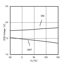
Fig.18. STB threshold temperature property
