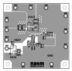
The radiation plate on the rear should be a GND flat surface of low impedance in common with the PGND flat surface. It is recommended to install a GND pin in another system as shown in the drawing without connecting it directly to this PNGD. Produce as wide a pattern as possible for the VBAT, Lx and PGND lines in which large current flows.
