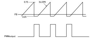
When voltage difference between input and output voltage is large and output current is small, DCDC converter switches as this non-synchronous mode then ripple voltage of output voltage could be large.
