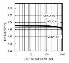
Fig.34 Load regulation (VOUT = 1.2 V)
