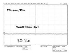
Fig.46 Output ripple 3 (VCC=12V, Io=140mA)
