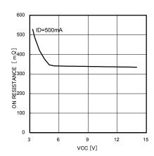
Fig.11. Nch FET ON resistance power supply property
