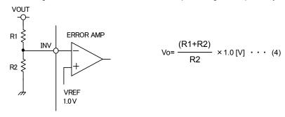
Fig.50 Setting of voltage feedback resistance
