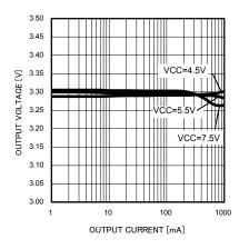
Fig.23 Load regulation (VOUT = 3.3 V)
