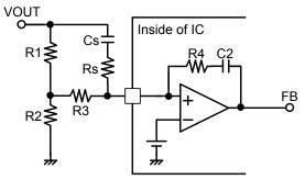
Fig.51 Example of phase compensation setting
