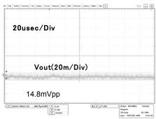
Fig.48 Output ripple 5 (VCC=12V, Io=900mA)
