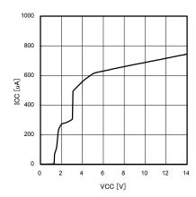
Fig.20. Circuit current voltage property
