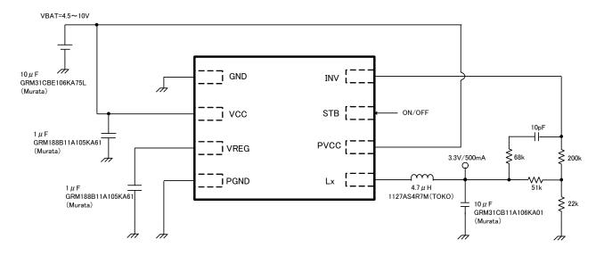
Fig.21 Reference application diagram1
