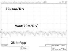
Fig.45 Output ripple 2 (VCC=12V, Io=100mA)
