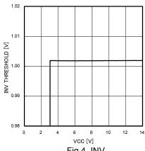
Fig.4. INV threshold power supply property
