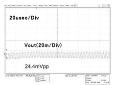
Fig.44 Output ripple 1 (VCC=12V, Io=40mA)
