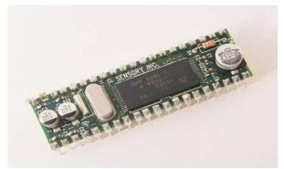
memory, Sensory's entire FluentChip™ library can be utilized including Record and Playback, along with lots of extended speech. The RPM is a prototyping tool designed for developers who will be creating product system designs that feature RSC-4x processor chips.
