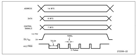
Figure 11. Programming Signal's Waveforms
