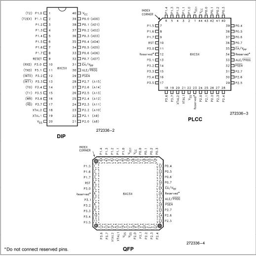
Figure 2. Pin Connections
