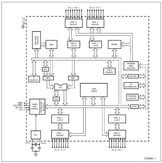
Figure 1. 8XC5X Block Diagram
