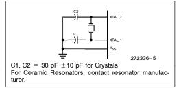
Figure 3. Oscillator Connections
