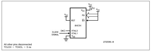
Figure 6. I<sub>CC</sub> Test Condition, Active Mode
