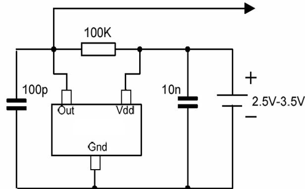
SEC's pole-independent sensing technique allows for operation with either a north pole or south pole magnet orientation, enhancing the manufacturability of the device. The state-of-the-art technology provides the same output polarity for either pole face. It is strongly recommended that an external bypass capacitor be
