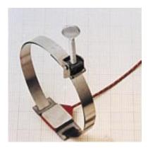
This 100R IEC 751 class B sensor has very fast response and is ideal for industrial control applications. The pipe clamp fitting allows a fast non intrusive installation. Other pipe clamp sizes can be made available up to 90cm diameter.
