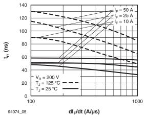
Fig. 5 - Typical Reverse Recovery Time vs. dI<sub>F</sub>/dt (Per Leg)
