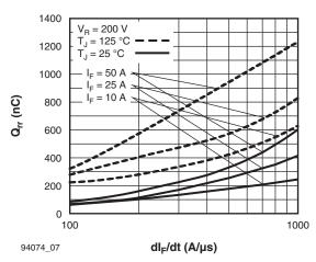
Fig. 7 - Typical Stored Charge vs. dl<sub>F</sub>/dt (Per Leg)
