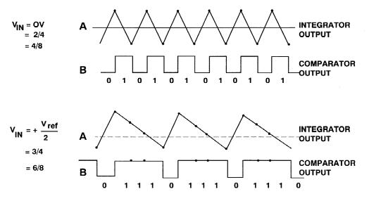
Figure 5: Sigma-Delta Modulator Waveforms
