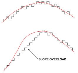
Figure 2: Quantization Using Delta Modulation
