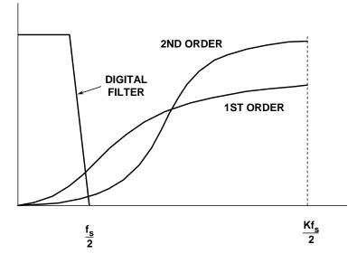
Figure 7: Sigma-Delta Modulators Shape Quantization Noise
