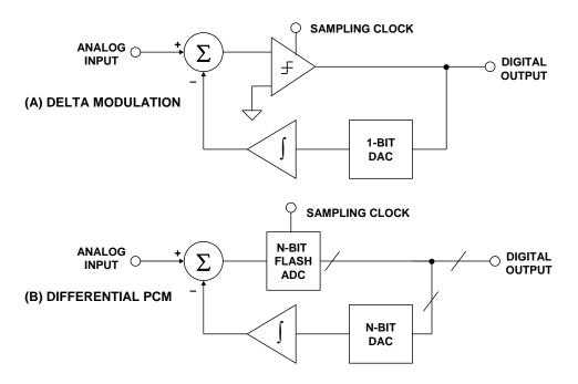
Figure 1: Delta Modulation and Differential PCM
