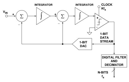
Figure 8: Second-Order Sigma-Delta ADC
