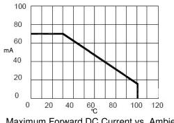
Maximum Forward DC Current vs. Ambient Temperature
