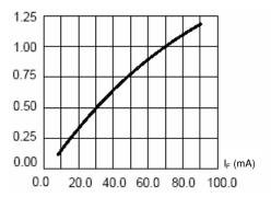
Relative Luminous Flux vs. Forward Current
