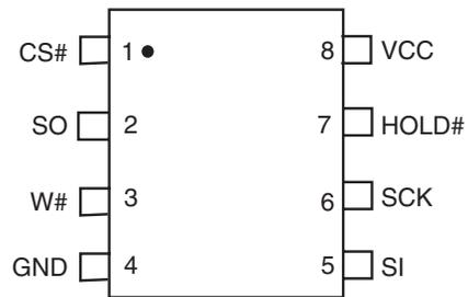
**Figure 2.2** 8L USON (5 x 6 mm) Package
