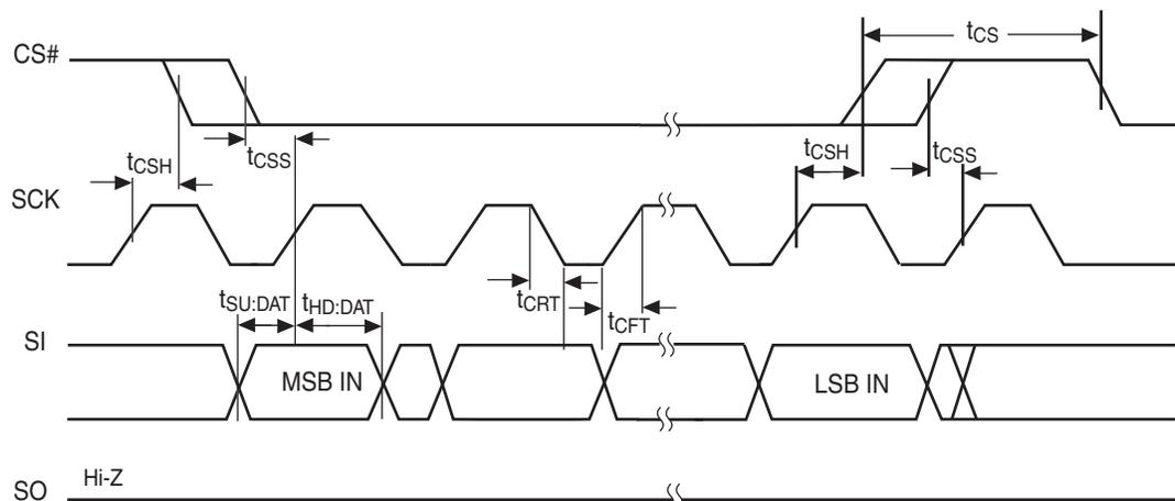
Figure 16.2 SPI Mode 0 (0,0) Output Timing
