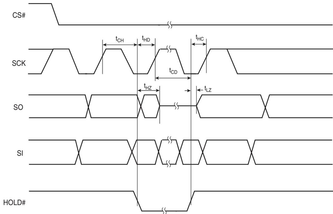
**Figure 16.4** Write Protect Setup and Hold Timing during WRSR when SRWD=1
