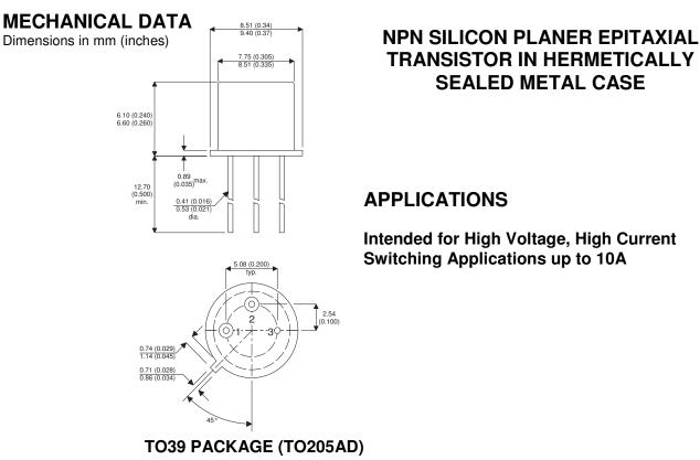
Pin 1 = Emitter Pin 2 = Base Pin 3 = Collector
