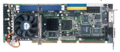
The HS-7002 is an Intel® 82865GV/82801EB chipset-based board designed for PICMG Bus PGA 478 Intel® Pentium® 4 CPU with speed of up to 3.2GHz CPU. The combination of these features makes the HS-7002 an ideal all-in-one industrial single board computer. Additional features include an enhanced I/O with CRT/LVDS Panel, TV-Out, dual Giga LAN, audio, serial ATA, 4 COM port interface, and more.
