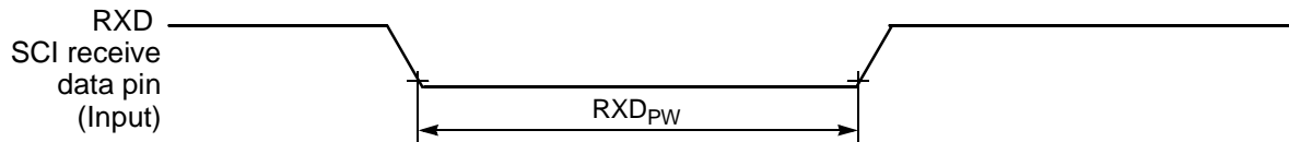
Figure 10-15 RXD Pulse Width
