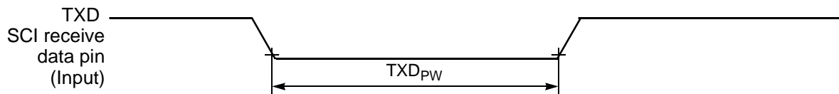
Figure 10-16 TXD Pulse Width
