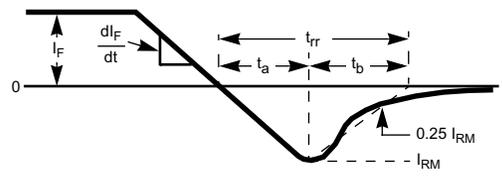
Figure 12.  $t_{rr}$  Waveforms and Definitions
