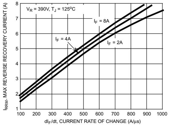
Figure 6. Maximum Reverse Recovery Current vs  $dI_F/dt$
