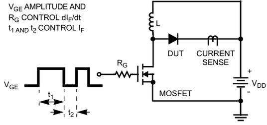
Figure 11.  $I_{t_{rr}}$  Test Circuit
