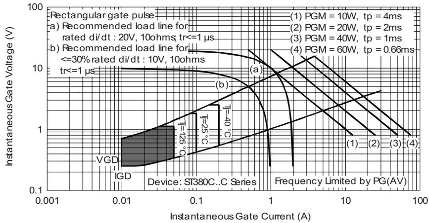
Fig. 11 - Gate Characteristics
