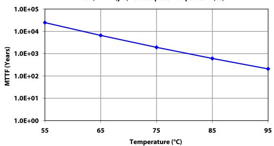
MTTF is calculated from accelerated life-time data of single devices and assumes isothermal back-plate.
