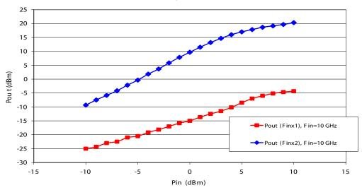
Measured results taken at room temperature in 40 GHz connectorized test fixture with no de-embedding.
