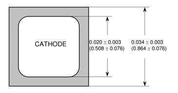
Bottom side metalization: Al - 25 kÅ minimum or Ti/Ni/Ag - 30 kÅ minimum.
