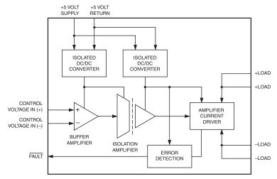
Figure 1. Simplified Schematic
