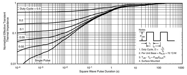
Normalized Thermal Transient Impedance, Junction-to-Ambient
