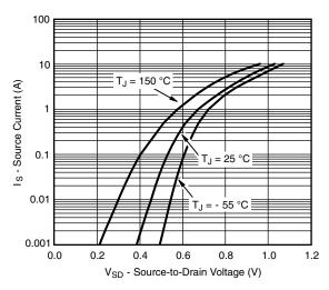
Source-Drain Diode Forward Voltage
