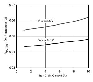
On-Resistance vs. Drain Current
