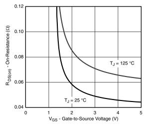
On-Resistance vs. Gate-to-Source Voltage
