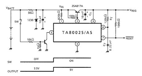
\*: Use an output capacitor C<sub>1</sub> which has a low temperature dependence (such as a tantalum capacitor) . Connect it as close to the IC as possible.
