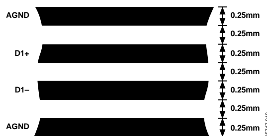
Figure 61. Arrangement of Signal Tracks
