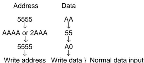
The SDP mode is disabled by inputting the following 6 bytes code. Note that, if data is input in the SDP disable cycle, data can not be written.
