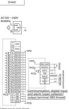
Digital input and alarm (open collector) output terminal, D-Sub terminal
