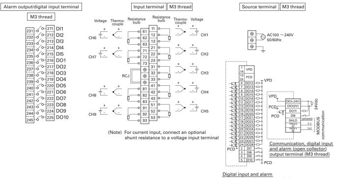
(open collector) output terminal, D-Sub terminal
