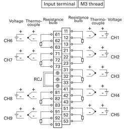
(Note) For current input, connect an optional shunt resistance to a voltage input terminal
