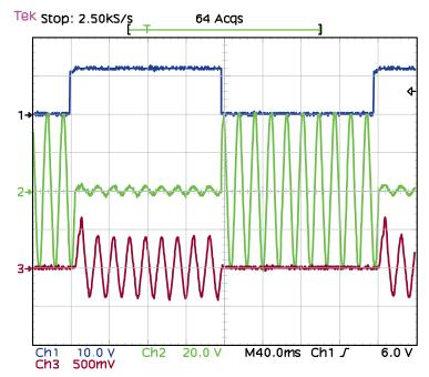
**Channel 1:** EN signal 0 to 12V logic input turning the solenoid on and off.
