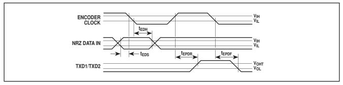
Figure 9 - Encoder timing parameters
