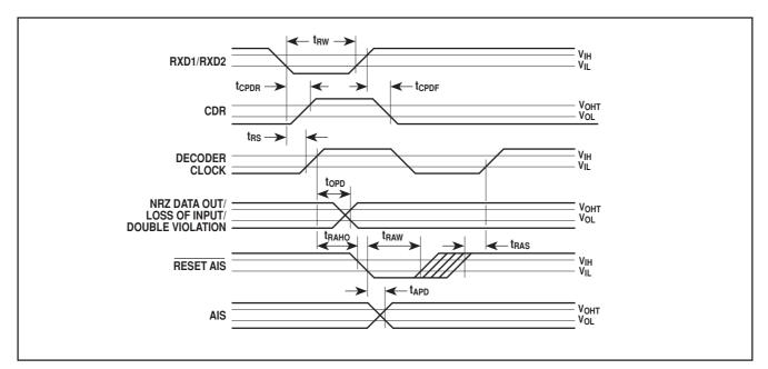
Figure 10 - Decoder timing parameters
