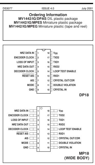
Figure 1 - Pin connections - top view
