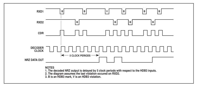
Figure 4 - Decoder waveforms
