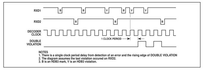
Figure 5 - HDB3 double violation waveforms
