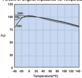
Measured on a 2661000301 using the HP4291A.
