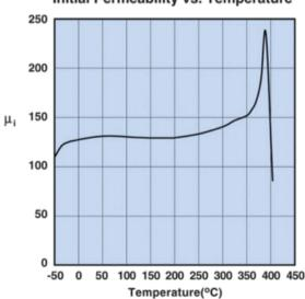
Measured on a 19/10/6mm toroid at 100kHz.
