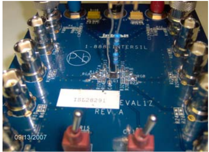
FIGURE 8. IMPROVED ANTENNA DESIGN TO EVALUATE RADIATED INTERFERENCE
