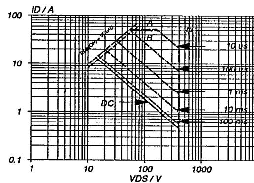
Fig.4. Safe operating area.  $T_{mb} = 25^\circ\text{C}$
