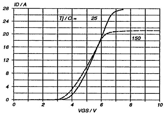
Fig.8. Typical transfer characteristics.
