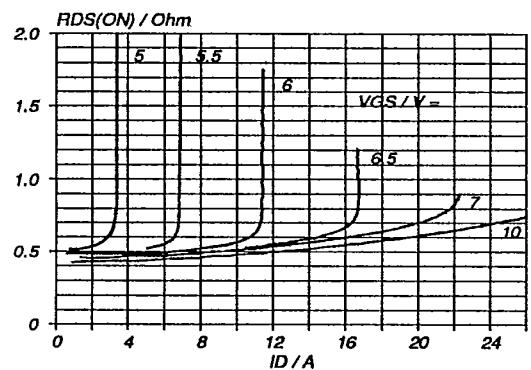
Fig.7. Typical on-state resistance,  $T_j = 25^\circ\text{C}$ .
