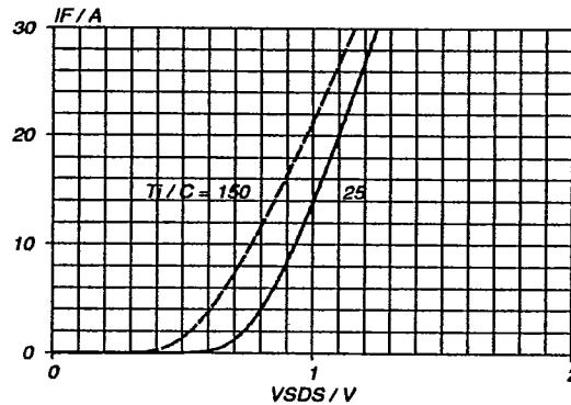
Fig.15. Typical reverse diode current.
