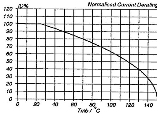
Fig.3. Normalised continuous drain current.
