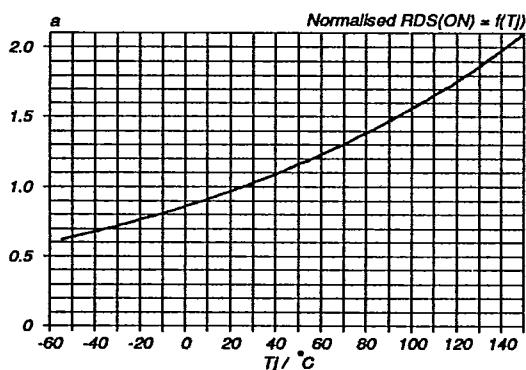
Fig.10. Normalised drain-source on-state resistance.
