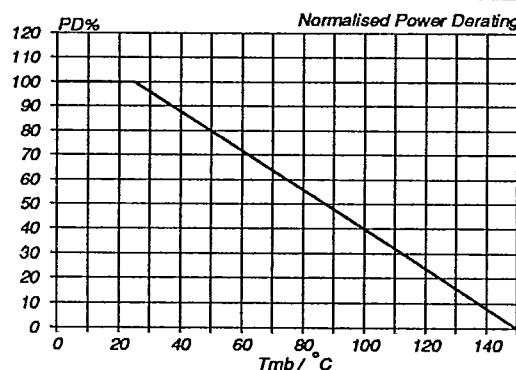
Fig.2. Normalised power dissipation.
