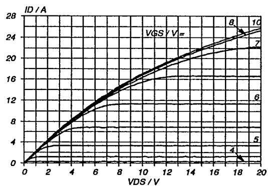
Fig.6. <sup>1</sup> Typical output characteristics,  $T_j = 25^\circ\text{C}$ .
