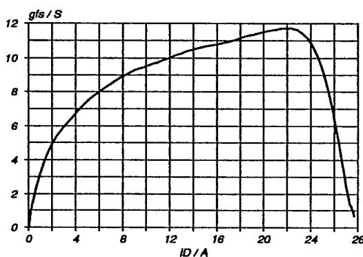
Fig.9. Typical transconductance,  $T_j = 25^\circ\text{C}$ .
