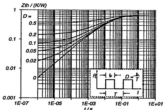
Fig.5. Transient thermal impedance.
