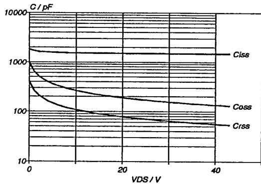
Fig.13. Typical capacitances,  $C_{iss}$ ,  $C_{oss}$ ,  $C_{rss}$ .
