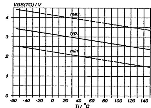
Fig.11. Gate threshold voltage.
