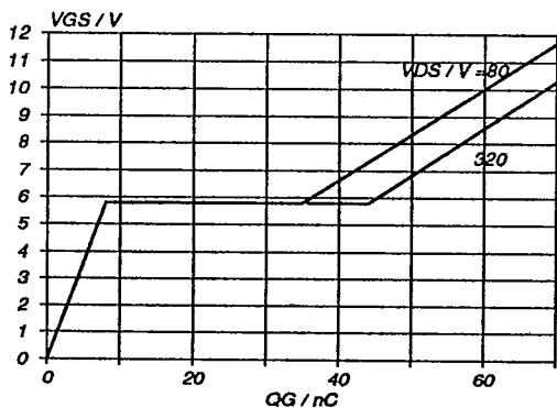
Fig.14. Typical turn-on gate-charge characteristics.
