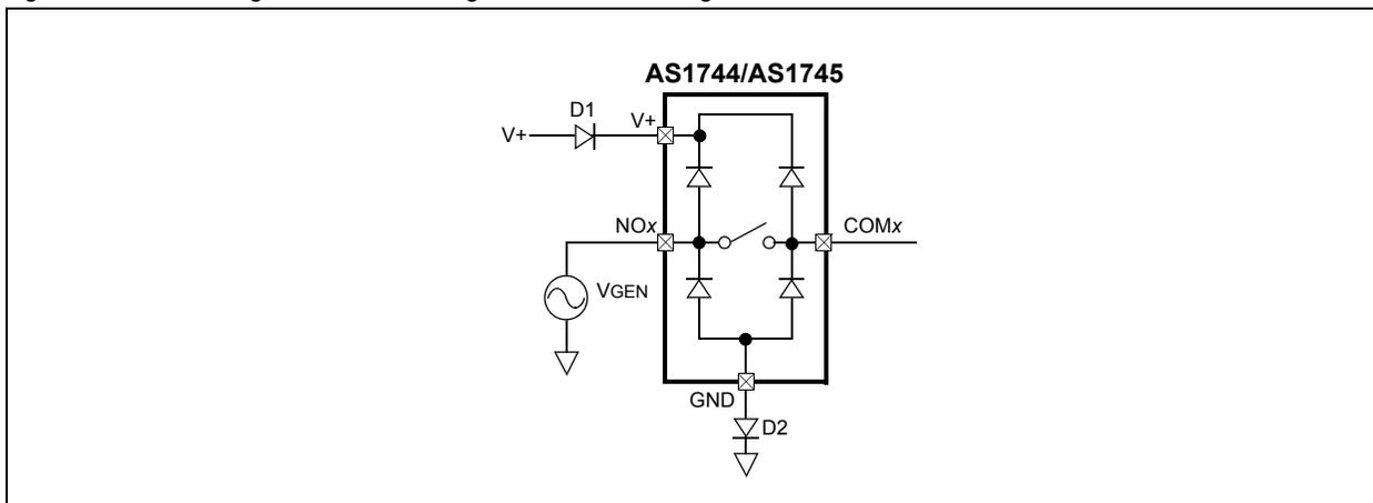
Adding diode D2 to the circuit shown in Figure 10 causes the logic threshold to be shifted relative to GND. Diodes D1 and D2 also protect against overvoltage conditions.
