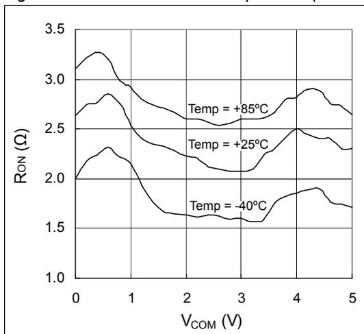
Figure 5. RON vs. VCOM and Temperature (VDD = 3V)
