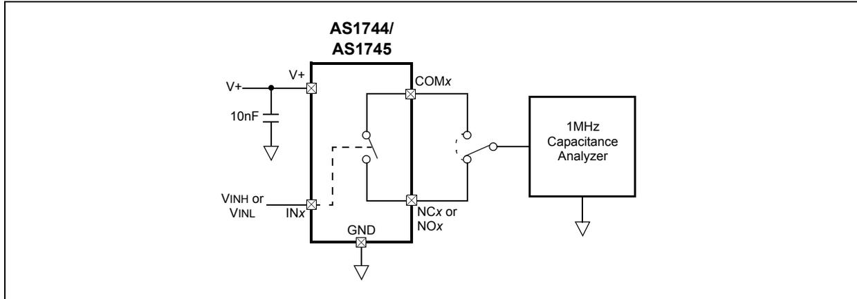
Figure 15. Off-Isolation, On-Loss, and Crosstalk
