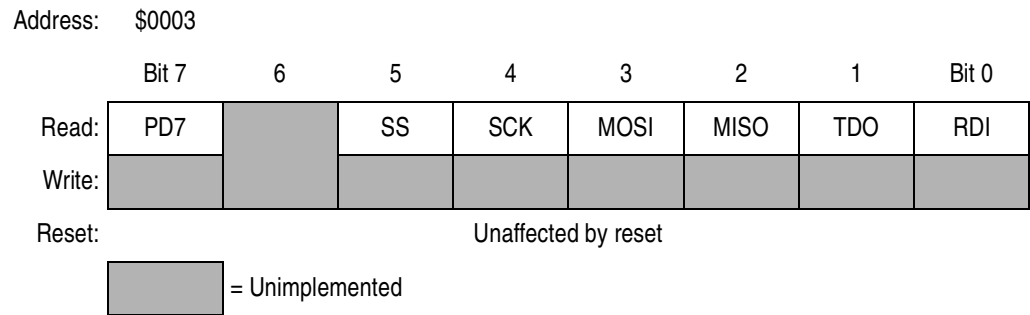
Figure 7-10. Port D Fixed Input Register (PORTD)
