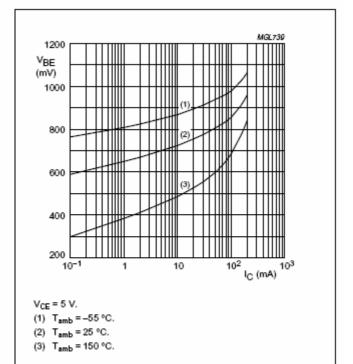
Fig.3 Base-emitter voltage as a function of
